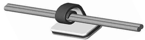
CORRECT! This method will keep wires off the surface of the instrument and hold them securely preventing unwanted vibrations.
